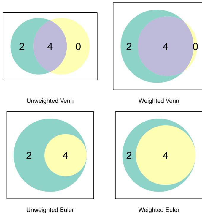
Figure 21: Effect of the doEuler and doWeights flags for a Venn object with Weights(V) [\"01\"] = 0
